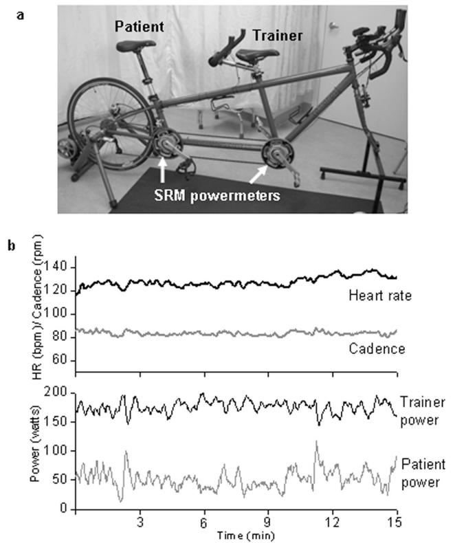
Note: a, A tandem bicycle was mounted on a mechanical trainer with the front fork secured. SRM cranks were installed at both the trainer (front) and patient (rear) positions. b, During this FE session the human trainer produced  $175 \pm 11$  watts of power and the patient produced  $54 \pm 17$  watts. Cadence and heart rate for the patient participants were  $83.2 \pm 1.7$  rpm and  $128.8 \pm 5.3$  bpm, respectively.
